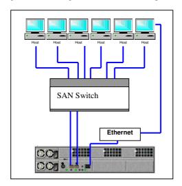
Note: For optimum performance, ensure that the HBA and SFPs used are 2Gb.
